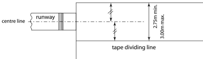
**Figure (b) TR29 (Rule 184) - Centralised Long Jump /Triple Jump landing area**
