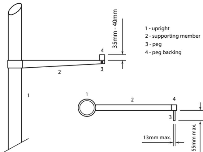
**Figure (b) TR28 (Rule 183) - Pole Vault crossbar support** (view from landing area and top view)
