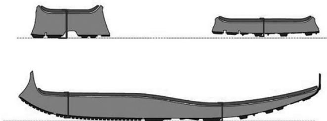
**Figure (a) TR5 (Rule 143) - Measuring the thickness of the sole**
